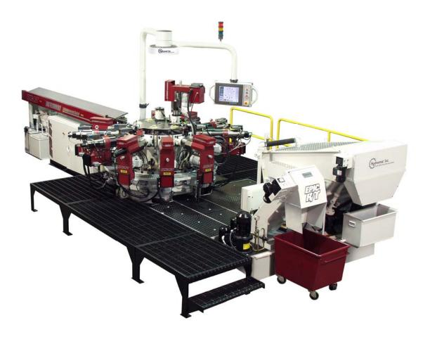
Caption: The EPIC R/T possesses all of the general characteristics of the more conventional Hydromat machines and maintains the integrity, reliability and flexibility of its predecessors. New EMC Technology (Embedded Motion Control) features special plug & play programmable CNC control components integrated into each toolspindle unit.
