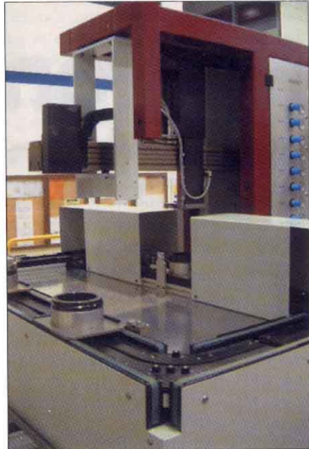
Typical parts that the AT machine is designed for include irregularly shaped cast or forged blanks within a 4" (100 mm) cube.
