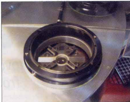
Erowa PowerChuck clamps pallet fixture with repeatability within two microns.
