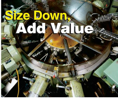
An overhead view shows the infeed tracks leading down to four tooling stations. Nuts are tapped in the Hydromat in four identical setups.
