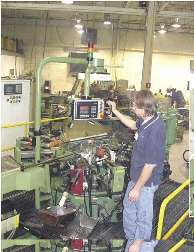
▲ When the tool monitoring system triggers a stop on this rotary transfer machine, an alert appears on the laptop display and also on the machine's pendant control (a red band is seen at the top of the display).
