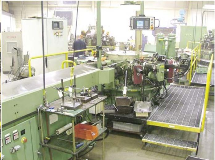
▲ The operator can devote more time to tasks away from the machine when he knows that the tool monitoring system will safely stop the machine if a tooling problem occurs.
