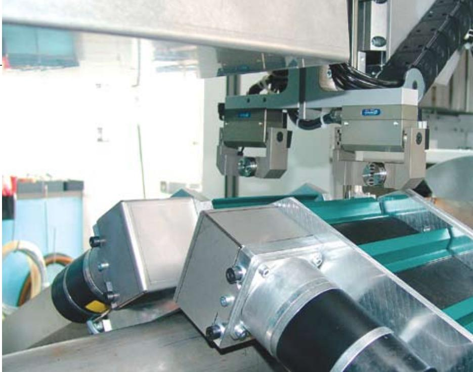
lematic with the addition of integral motors to the multi-spindle drum. Each motor is a source of heat, and with six or eight motors, an active system to help thermally stabilize the machine is necessary.
