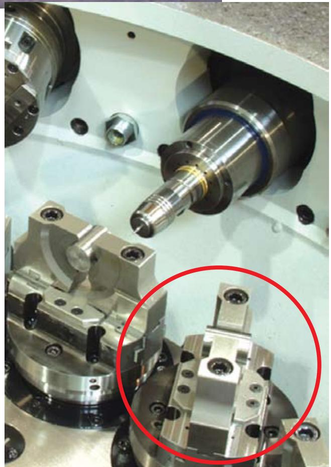
**For castings, forgings and other irregular blanks, custom clamping configurations can be engineered. ►**
