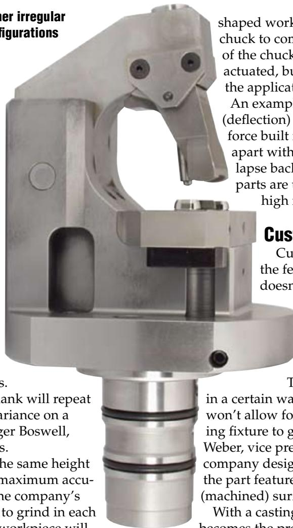
shaped workpiece is inserted into the second chuck to complete the transfer process. Most of the chuck jaws specified are hydraulically actuated, but other types may be used when the application requires them.
