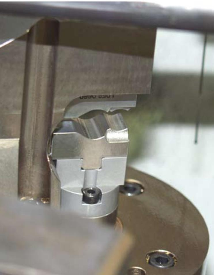
▲ To accelerate change-over for families of similar parts, inserts can be used in the indexing chucks. These are quick-change requiring only a new set of jaws and can be changed in an hour or less for all of the rotary transfer stations.
