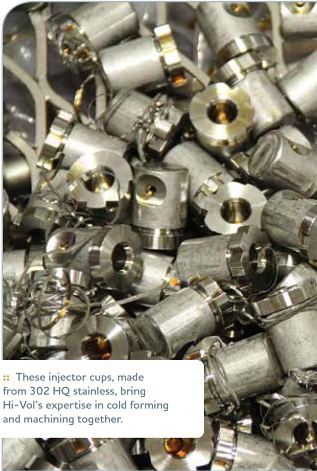
∴ These injector cups, made from 302 HQ stainless, bring Hi-Vol's expertise in cold forming and machining together.
