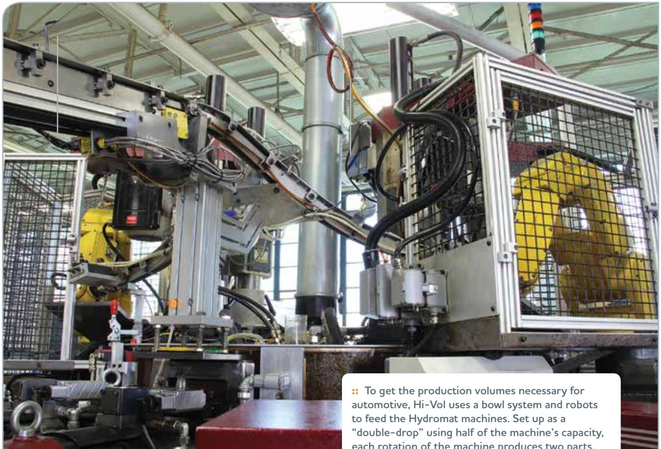
☺ To get the production volumes necessary for automotive, Hi-Vol uses a bowl system and robots to feed the Hydromat machines. Set up as a “double-drop” using half of the machine’s capacity, each rotation of the machine produces two parts.
