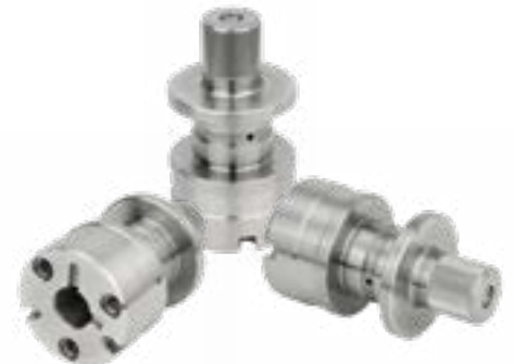
Ø 46x80mm - 1144 STEEL - BAR STOCK CYCLE TIME: 21.5 SEC
