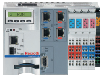
Rexroth IndraControl L85 Source: Bosch Rexroth AG
