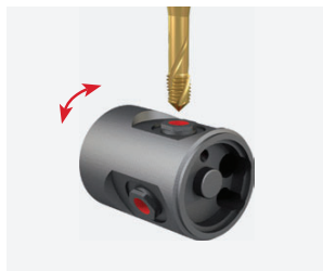
Station 6V, tool 1, turret Tapping
