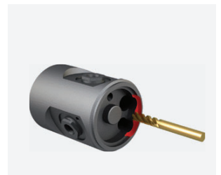
Station 6H, tool 1, turret Milling the recess
