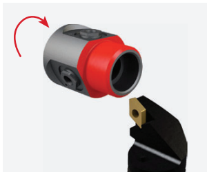
Station 10H, tool 1, Capto holder External turning
