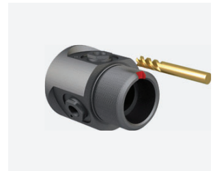
Station 11H, tool 1, turret Slot milling
