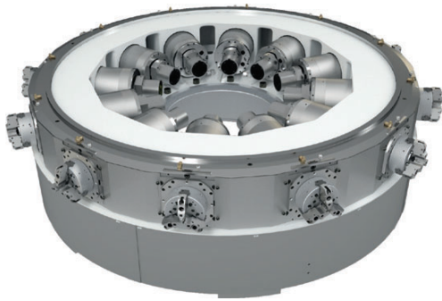
A look at the centrepiece, the rotary indexing table with 12 workpiece spindles
