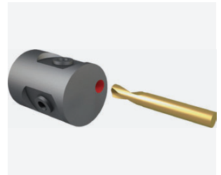
Station 2H, tool 1, turret Rough drilling
