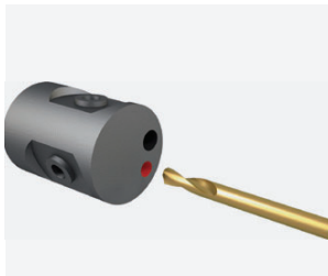
Station 2H, tool 2, turret Rough drilling
