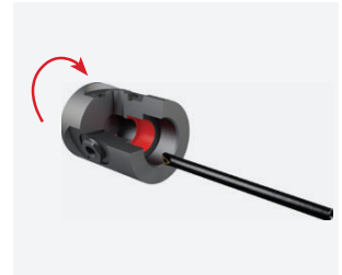
Station 9H, tool 4, turret Turning an inner contour
