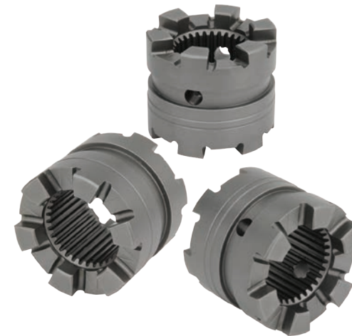
Ø 57.2mm - 4340 STEEL - BAR STOCK CYCLE TIME: 25.0 SEC
