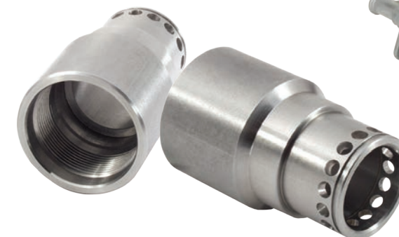
Ø 50x65mm - ALLOY STEEL - 1144 - BAR STOCK CYCLE TIME: 20.7 SEC
