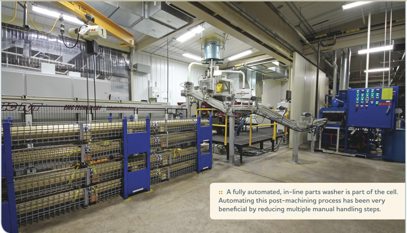
∴ A fully automated, in-line parts washer is part of the cell. Automating this post-machining process has been very beneficial by reducing multiple manual handling steps.
