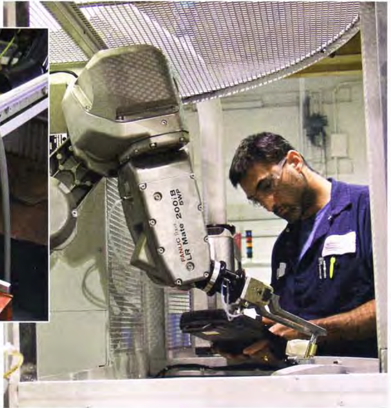
▲ Another aspect of the retrofit was installation of a robot for unloading the finished parts. Using the robot frees an additional station on the 12-station Hydromat. The robot deposits the finished parts on a conveyor (above). ▶
