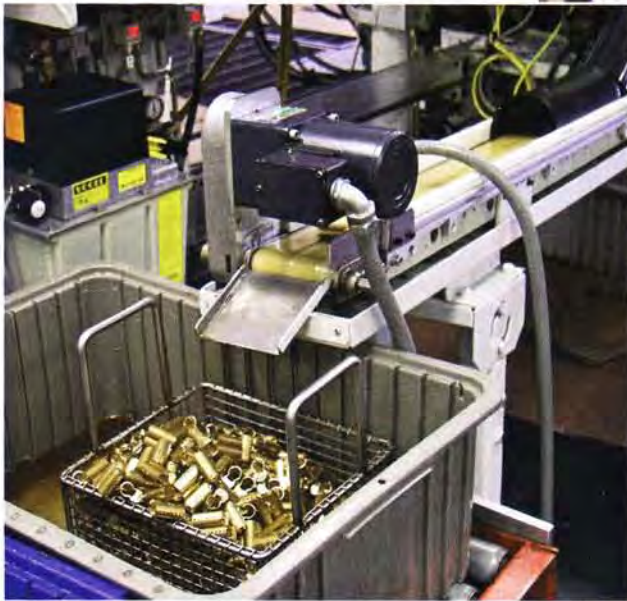
▲ Another aspect of the retrofit was installation of a robot for unloading the finished parts. Using the robot frees an additional station on the 12-station Hydromat. The robot deposits the finished parts on a conveyor (above). ▶
