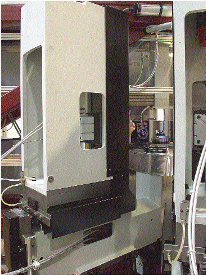
Key to 2-micron locating accuracy in Hydromat's AT rotary transfer machine is the cast C-frame modules. The pallets rest on the frame itself. The indexing table simply lifts the pallet from the frame, moves it to the next station, and inserts it into the coupling in that module's frame
