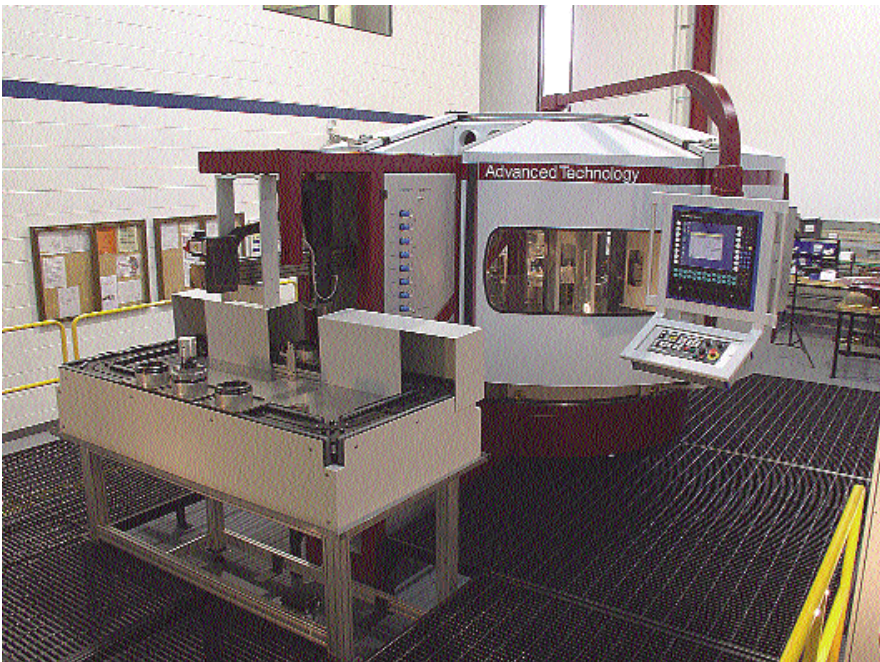
To streamline loading, Hydromat's AT flexible rotary transfer machine comes with a staging table, on which the operator places preset fixtures. Once the machine indexes, a pick-and-place unit removes the pallet containing the finished piece from the table's loading station and inserts a new pallet
