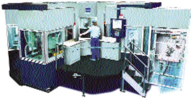
Like other hybrids, Kirby's Rotoplan reduces costs over banks of machining centers by eliminating queues and setup and needing only one operator to run the equivalent of as many as eight machining centers
