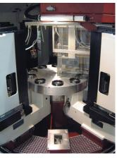
On Hydromat's new AT machine, the table lifts and rotates to index the workpieces from station to station. The machining units are modular and can be set up off-line to expedite changeover from job to job.
