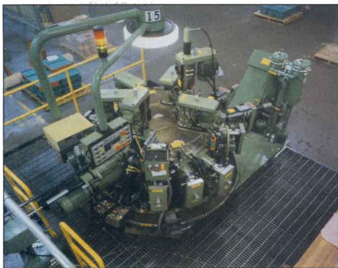
The HB 32/45-16 is a 16-station rotary machine that produces delicate, close-tolerance parts at high cycle times.
