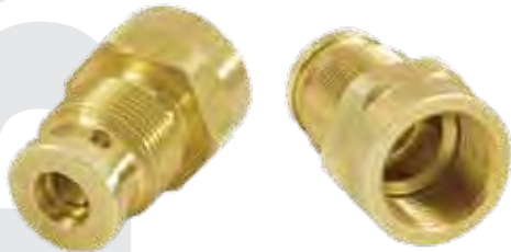
BRASS - 360 - BAR STOCK CYCLE TIME: 7.5 SEC
