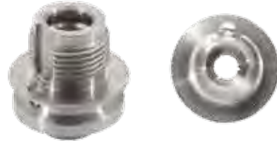
FREE MACHINING STEEL - 12L14 - BAR STOCK CYCLE TIME: 9.0 SEC
