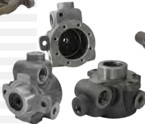
AUTOMOTIVE NODULAR IRON - CASTING CYCLE TIME: 110.0 SEC
