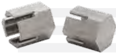
STEEL - 12L14 - BAR STOCK CYCLE TIME: 5.0 SEC
