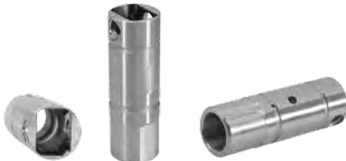
STEEL - 1013 - COLD FORMED BLANK CYCLE TIME: 5.1 SEC
