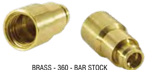
BRASS - 360 - BAR STOCK CYCLE TIME: 4.5 SEC
