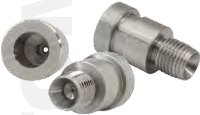
STAINLESS STEEL - 2205 - BAR STOCK CYCLE TIME: 17.0 SEC
