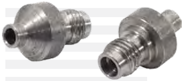
STAINLESS STEEL - 303 - BAR STOCK CYCLE TIME: 6.0 SEC
