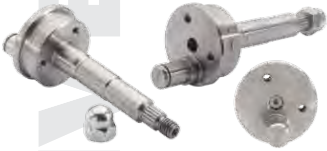
ALLOY STEEL - 8620 - PRE-MACHINED BLANK CYCLE TIME: 7.9 SEC
