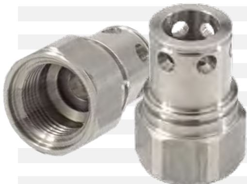
STAINLESS STEEL - 316 - BAR STOCK CYCLE TIME: 20.0 SEC
