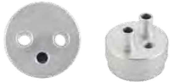
ALUMINUM - 6061 - BAR STOCK CYCLE TIME: 9.3 SEC
