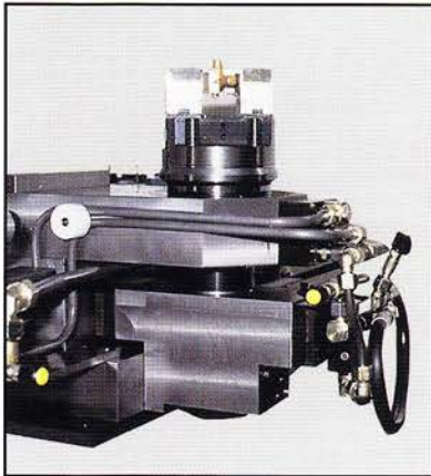
The hydraulic control for the indexing chucks is modular and can be incorporated at any station.
