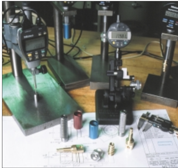
“We run 60 percent steel, 35 percent aluminum and 5 percent brass,” Barrie says. The steels are 12L14, 12L15, 1144 stress-proof and 1144 fatigue-proof. Every part is of a different material, or at least a different diameter of the same material.
