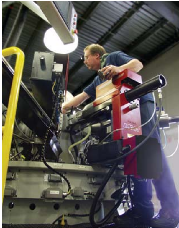
Comer concentrates on setting up the EPIC R/T 12. EPIC's program will let the technician know when it's time to change a tool.
