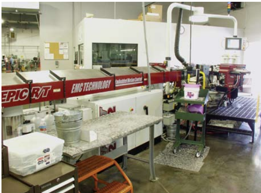
This reverse angle shows the parts conveyor for the EPIC R/T.
