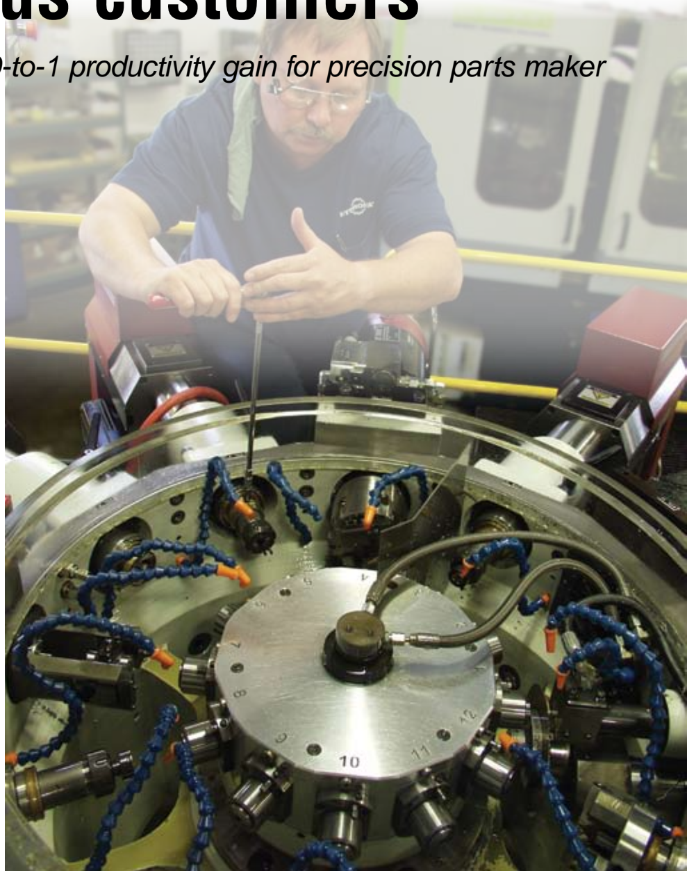
Lloyd Comer, supervisor of the rotary transfer department, ratchets up another changeover on the EPIC R/T 12.
