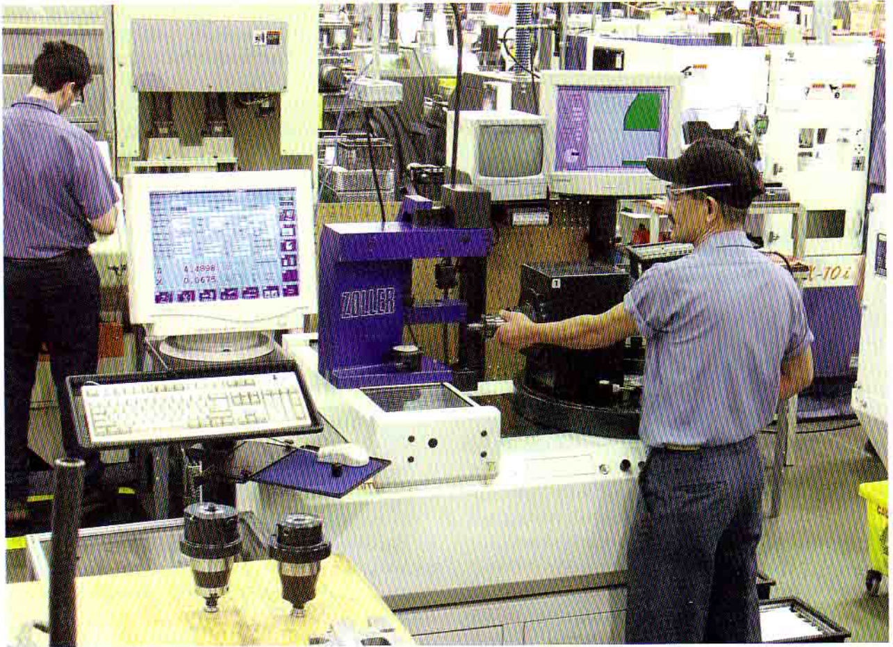
An optical tool presetter at the rotary transfer machines enables the operator to make fast, accurate tool changes.
